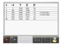
When the Straightness Target Value function is selected the Target Values are shown in the list (instead of notes).
