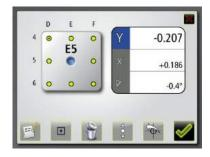
When a measurement point is registered, fixed values are indicated without a green vertical line beside the values.
