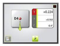
The actual Y value for the selected point goes live and alignment can be made towards zero. Zero will be in accordance to selected references.
