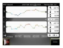
The screen displays measurement results, distances\*, tolerance, references, file name, date and time, serial number of the display unit and the sensor, program and program version.
