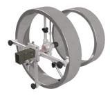
Adjust the laser transmitter so that the laser beam hits the centre of the target.  Move the receiver to the last bore.
