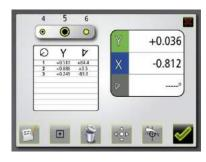
When the Arc Angle measurement is finished, a list of the values at each position is shown together with the result. This list will not be saved but it is possible to take a screen dump of it.
