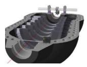
Adjust the angle of the laser beam, horizontally and vertically, by using the micrometer screws on the laser transmitter to position it in the centre of the second reference bore. Use a tape measure to position the beam into the centre within I-2 mm. 4. If necessary, repeat the procedure for coarse adjustment until the beam is centred in both reference bores.
