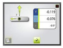
The actual values for the selected point go live and alignment can be made towards zero. Zero will be in accordance to selected references.
