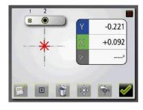
When a measurement point is registered, fixed values are indicated without a green vertical line beside the values. The colour indicates the status of the Y and X values in relation to the selected tolerance.
