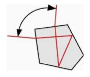
The built-in angular prism works as shown to the left. The incoming laser beam is deflected  $90^{\circ} \pm 0.02$  mm/meter also if the beam hits the prism obliquely.
