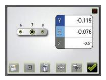
Place the receiver on the point. Make sure that the laser beam hits the target.
