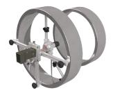
Rotate the receiver and the probe 180° and slide it to correct half of the difference between the laser spot and the centre.
