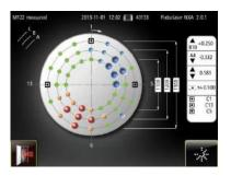
The screen displays measurement results, diameters, number of points on a circle, tolerance, references, file name, date and time, serial number of the display unit and the sensor, program and program version.
