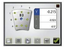
When a measurement point is registered, fixed values are indicated without a green vertical line beside the values.
