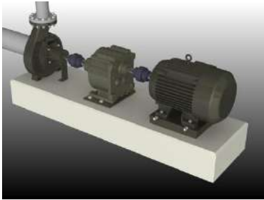
Machine Train with 3 machines.
