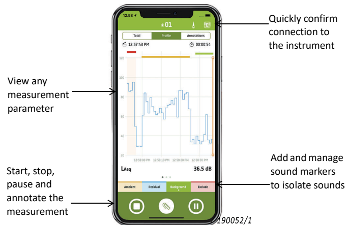
Fig. 2 Control, view and annotate measurements directly from your mobile device
